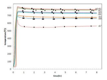
Figure 13. Temperatures measured with time at 0° inclination angle.
