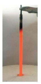
Figure 5. Heat pipe test at 800 °C.
