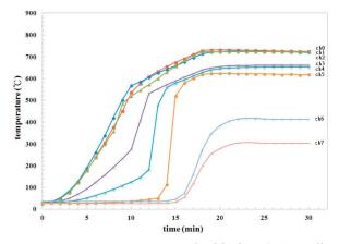
Figure 7. Temperatures measured with time (10% sodium filled, thermosyphon without wick).
