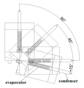
Figure 10. Schematics of different inclination configurations.
