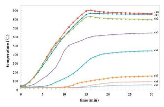
Figure 6. Temperatures measured with time (0% sodium filled, empty tube).
