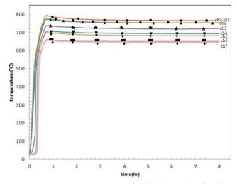
Figure 11. Temperatures measured with time at +90° inclination angle.
