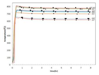
Figure 12. Temperatures measured with time at +45° inclination angle.
