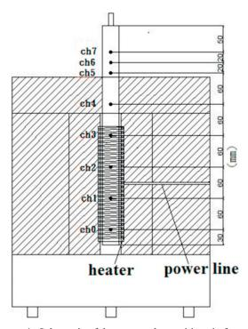
Figure 4. Schematic of thermocouples positions in furnace.
