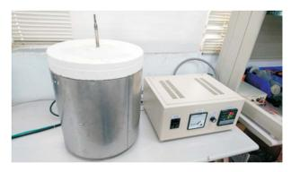
Figure 3. Heat pipe in furnace and power supply.
