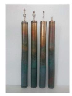
Figure 2. Heat pipes charged with sodium and sealed.
