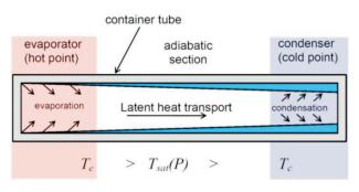
Figure 1. General heat pipe schematic diagram.
