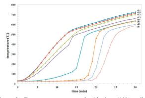
Figure 8. Temperatures measured with time (10% sodium filled, heat pipe with screen wick).
