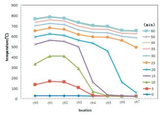
Figure 9. Transient axial temperature profiles along a heat pipe during a frozen startup period.
